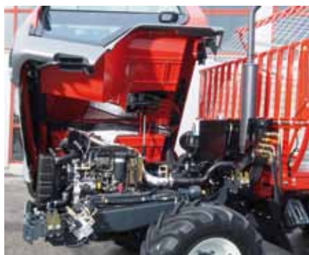
Technik-Highlight kippbare Komfortkabine
