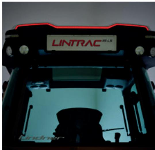
Powerful H7-halogen or LED working lights are available on request. For municipal use extremely visible LED rotating beacons and flash bars are used. For special operations LED roof flashers are used to increase the attention. They can be integrated perfectly into the TracLink roof shell – without disadvantages regarding the construction height.
