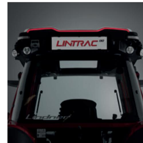
Upon request, powerful H7 halogen or LED working lights are also available. For urban applications, highly visible LED warning beacons and flashing light strips are used. In order to call attention to special operations, LED flashing light strips are employed which can be integrated perfectly into the TracLink roof shell - without negatively affecting the overall height.
